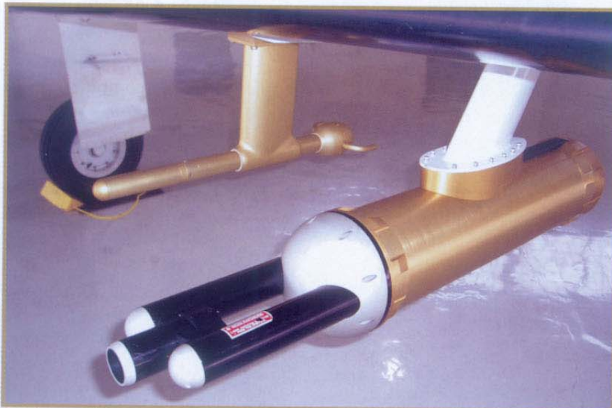
Another configuration option for the Cheyenne's left hardpoint pairs the Aventech Research AIMMS-20 with the FSSP by Particle Measuring Systems.
